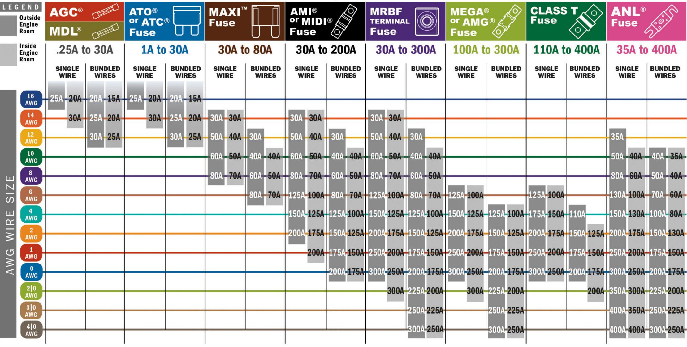
Although this process uses information from ABYC E-11 to recommend wire size and circuit protection, it may not cover all of the unique characteristics that may exist on a boat. If you have specific questions about your installation please consult an ABYC certified installer.
